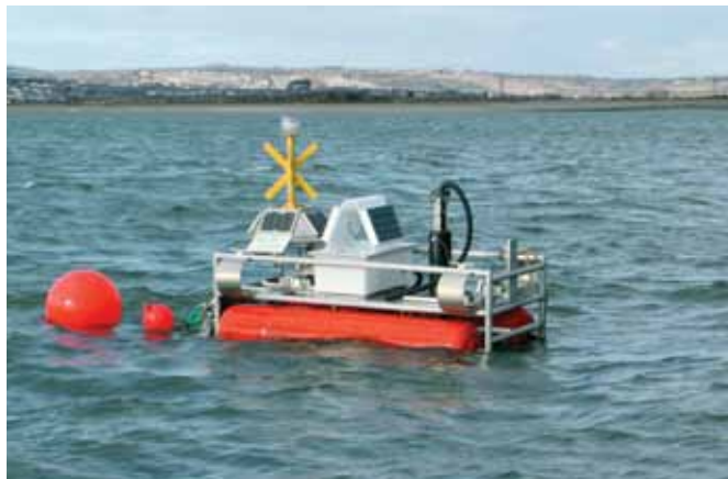
A customised pontoon supports water-quality instrumentation and power supplies for remote monitoring in high-flow zones.
