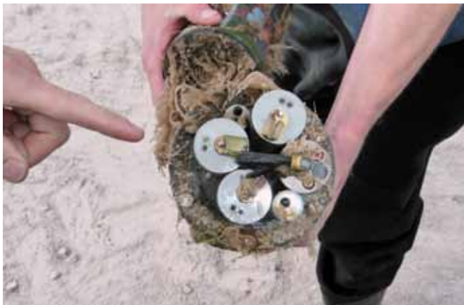
Even though the water-quality sonde is deployed for months, anti-fouling features keep the sensors clear of biofouling.
